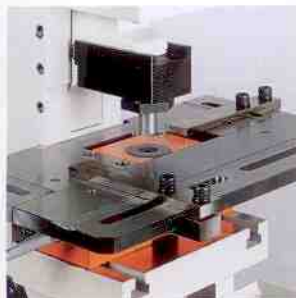
*Punching tool on notching station.
